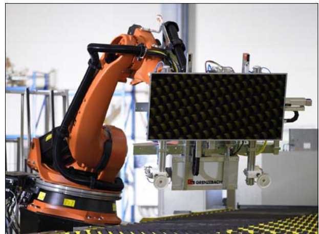
Robots by Grenzebach Maschinenbau GmbH are responsible for handling the production process of thin film solar modules
