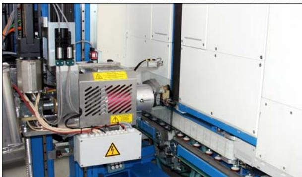
This robot developed by Lenhardt Maschinenbau GmbH is core to the machinery used in the production of thin film solar modules totally free of laminate
